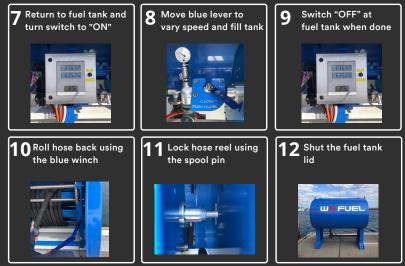
Please note: After 15 seconds of inactivity the hose will cut out and you will have to begin the process again by reactivating a transaction at the Smart Fuel Terminal.
