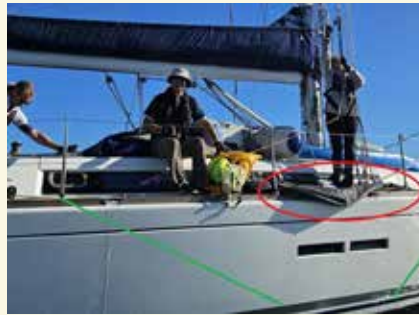
Papillon : Shade cloth wrongly positioned - Red Circle versus intended deployment - Green Lines
