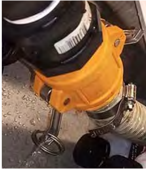
Camlock wings down – fitting open.
